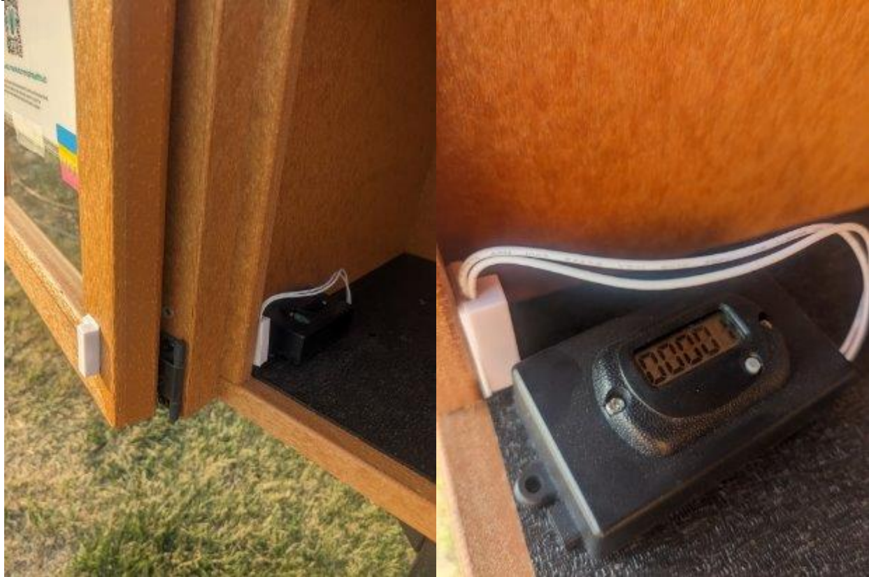
Figure 4: Magnetic counter placed on the inside door of the library to track how many times the door is opened.
